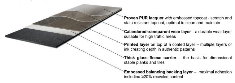
Figure 1: Typical construction
