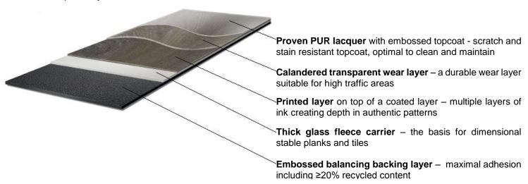
Figure 1: Typical construction
